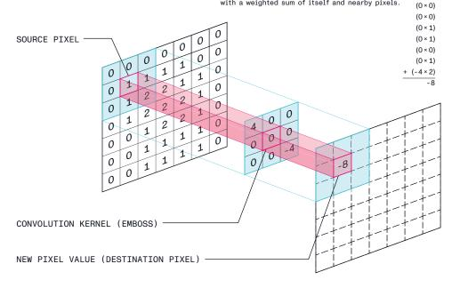
23. Diagram of a convolution, a filter applied to a small part of an image, in a convolutional neural network
